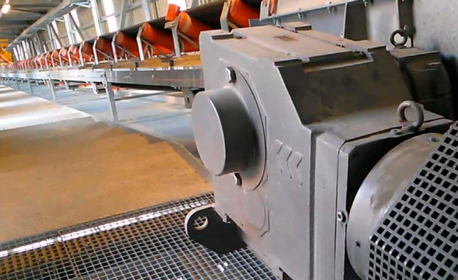
Figure 2: The inclined conveyor belt with Watt Drive technology transports the bulk material to the reversible belt, which deposits the bunker material.
